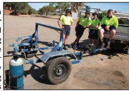
without the need of hydraulics or a tractor. This means that it can be towed with our normal dual cab utes and still be unrolled in the paddock. This is very nearly finished and the next decision is what colour to paint it.
